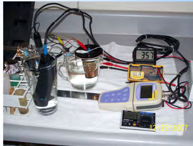
Experimental setup with electrode assembly partially immersed in 300 mls seawater. Voltage, amperage, pH, and time readouts on right. pH probe on left.
