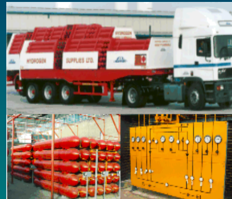
Tube Trailer delivery and storage modules
