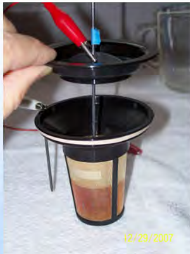
Electrode assembly with graphite anode inserted into porous cup containing powdered \text{CaCO}_3 .
