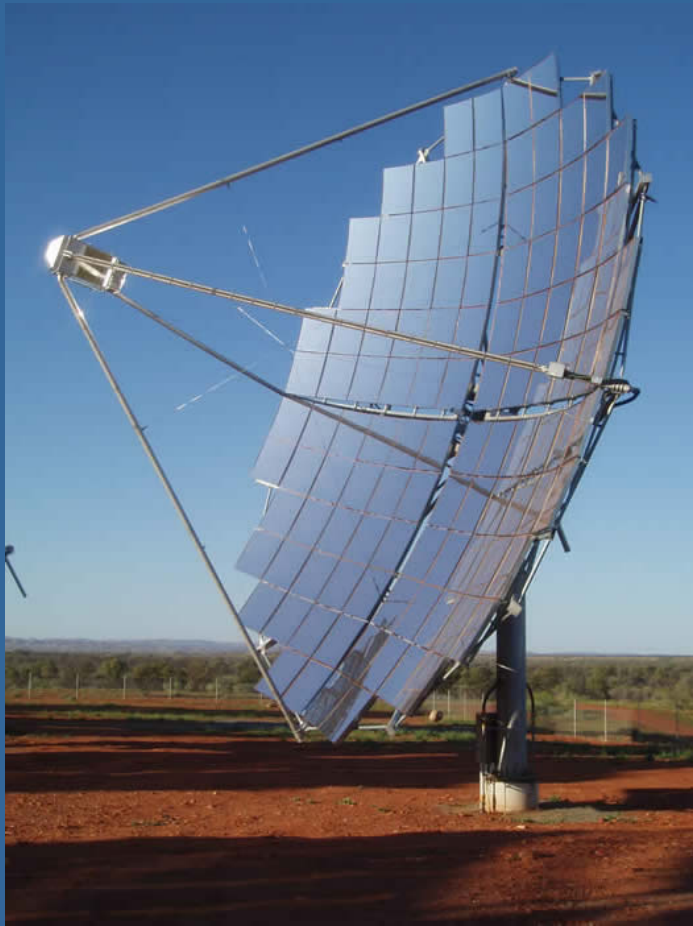
Solar Systems 35kW PV reflective concentrator
